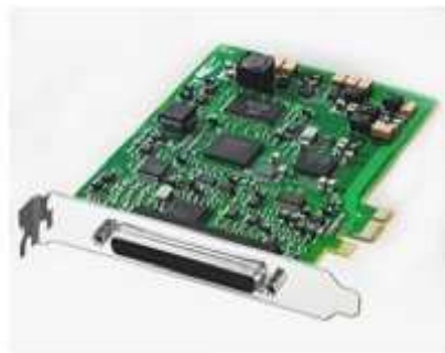
Standard Definition (SD) 10-bit video capture card -- Blackmagic DeckLink SD is pictured, Mac or PC; 12-bit cards also.
